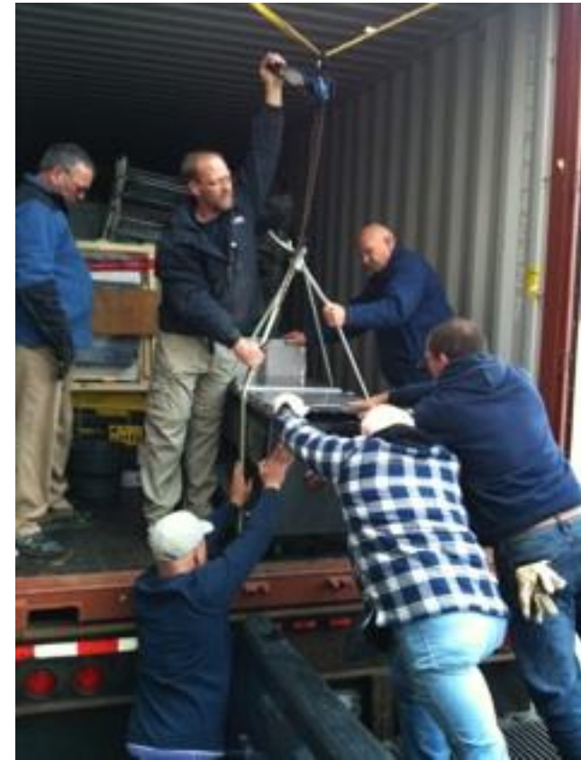
This surgical table weighed 800-900 pounds, and needed a block-and-tackle to lift it.
