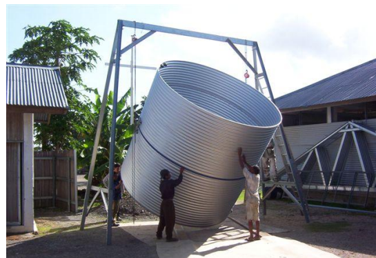
A 27,000 litre tank for the island of Ata Uro, the largest made by ETRP
